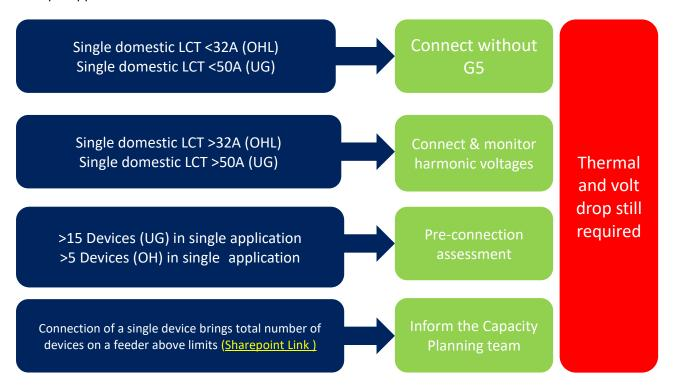
If the multiple application consists of identical heat pumps, the conditional connection assessment required by BS EN 61000-3-11 may be carried out for the installation with the highest source impedance only. Similarly, the BS EN 61000-3-12 assessment may be carried out for the PCC with the lowest fault current only.
