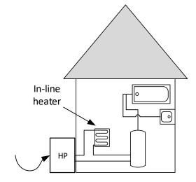
Air-to-water HP unit with inline heater
