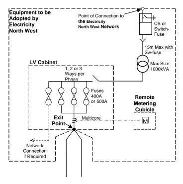
Figure 2 – Connection with NO Provision for LV Network
