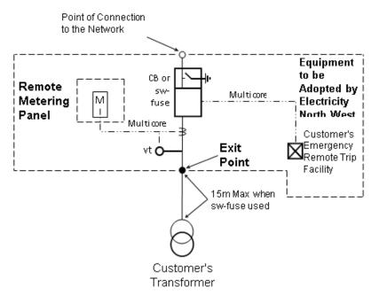
Figure 2 Connection with NO Provision for LV Network
