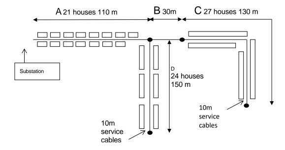
All 72 houses have electric heating on an unrestricted tariff and so the ADMD is 3.4kW for each property. Distributed loads are considered as concentrated at the mid-point of the section to which they are attached.
